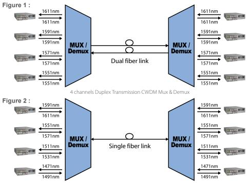
4 channels Bi-Directional Transmission CWDM Mux & Demux
