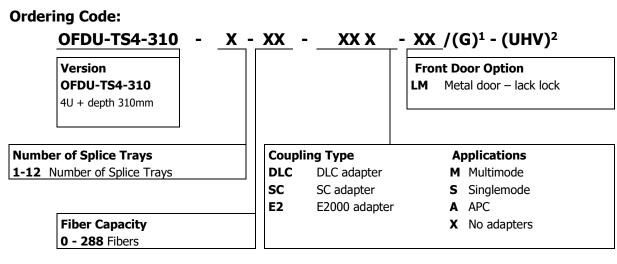
NOTE: 1) G - Grounding option - Protection grounding wires installed, see datasheet CMS\_01-02\_EN-accessories 2) UHV - Vertical unit holder-optional
