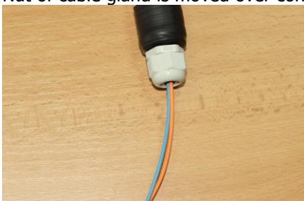
Nut of cable gland is moved over connectors
